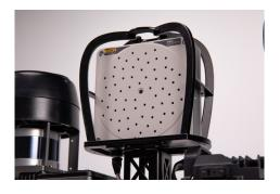
Acoustic imaging is a newer leak detection method that picks up audible and visual indicators of a leak. Workers scan equipment with an ultrasonic sensor to see if it picks up a signal. The exact location of the leak can be pinpointed as the signal gets stronger the closer the sensor gets to it. While basic ultrasonic sensor is not very precise—the signal is easily corrupted by nearby ultrasound-emitting equipment for example, acoustic imaging leverages beamforming to cut through the noise.
