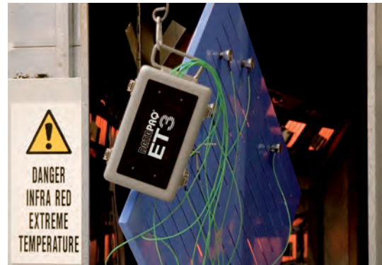
Fig. 1 The thermal barrier protects the data logger as it moves through the oven or furnace.
